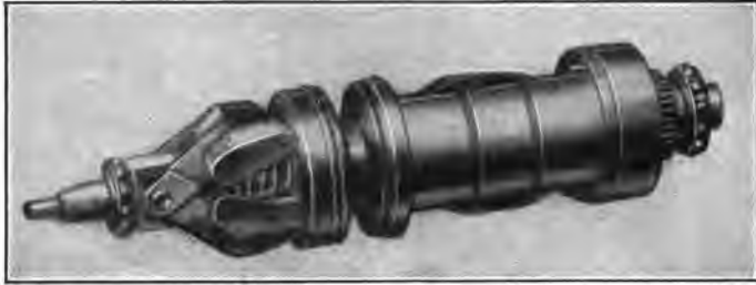
FIG. 153.—Eisemann armature with automatic spark advance mechanism.
